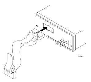
**4** Plug the keyed end of the cable (pin 14 is blocked) into the JTAG debug port on the target system.
