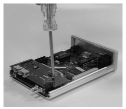
**4** Remove the 3 nylon screws from the target board adapter.
