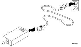
**3** Connect the 12V power cord to the back of the emulation probe.
