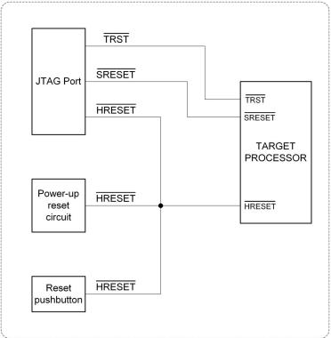
The emulation probe adds capacitance to all target system signals routed to the JTAG debug port connector. This added capacitance may increase the rise time and/or fall time of the reset signals beyond target processor specifications. Decreasing the value of the pull-up resistor on a line will decrease its rise time.
