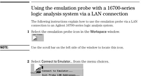
**3** Enter the emulation probe's LAN name or IP address and select the **Connect to Emulator** button.
